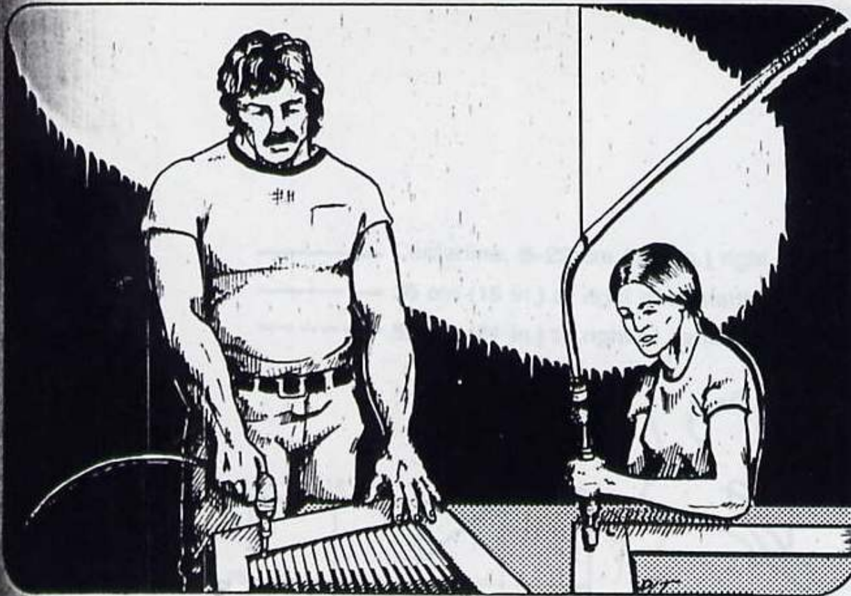
Figure 27. Shows the effects of being seated or standing on the type of tool handle needed to maintain a straight wrist.
