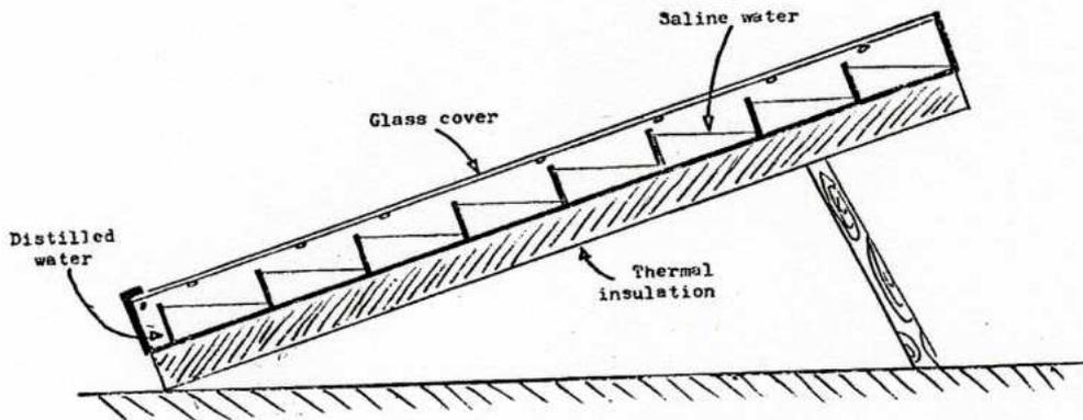
FIG. 2 - Tilted solar still with metal tray.
