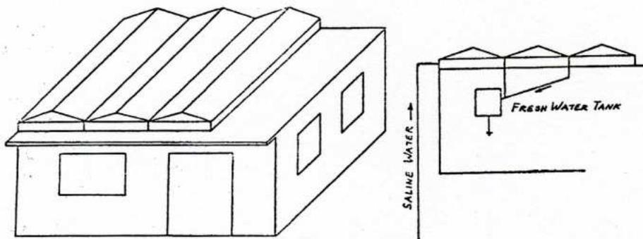
FIG. 3 - Design of a concrete solar still to be placed on the roof of houses in arid zones.
